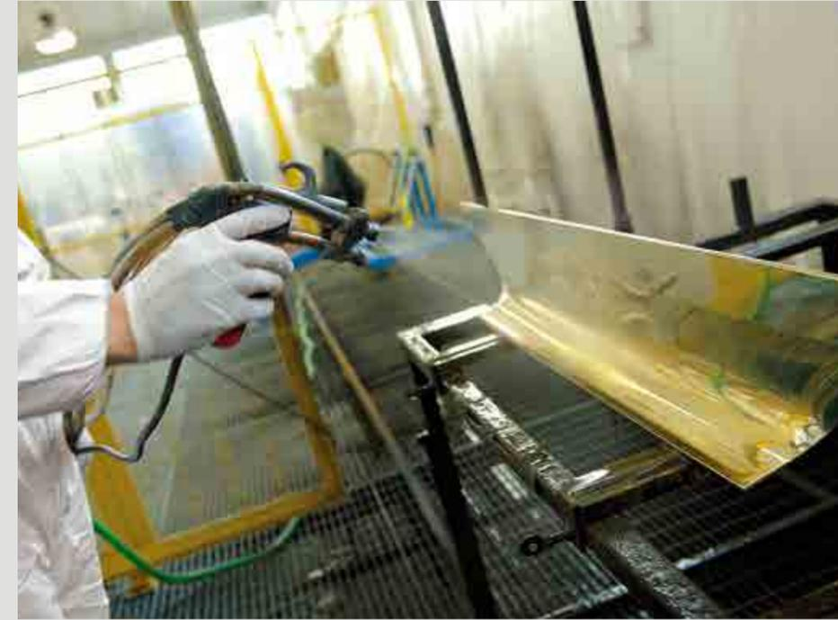
This process consists of depositing metallic silver (through the precipitation of silver nitrate) on the parts not in contact with the tin, and allows the creation of glass with the ability to reflect any rays of light that strike its surface.
